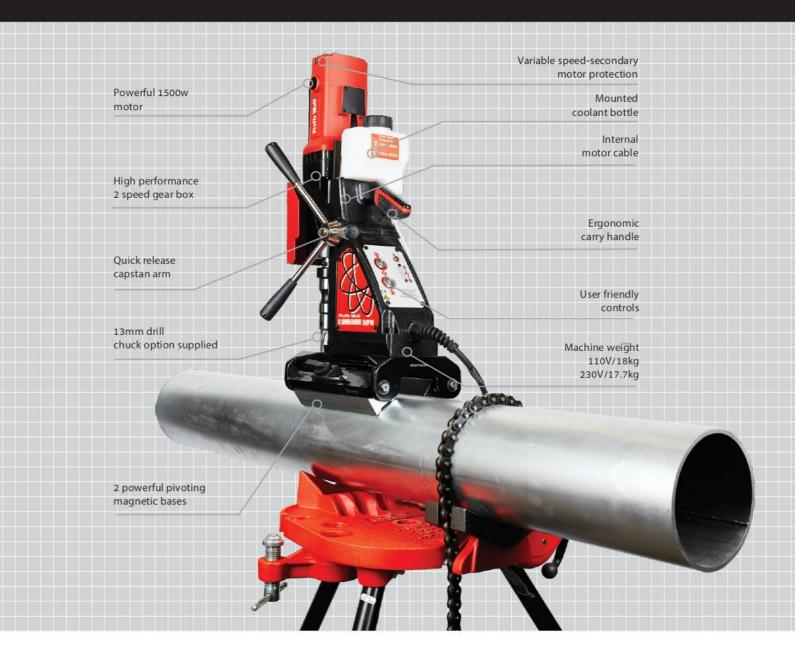
The latest addition to the Ralliwolf range, the COMMANDO 50 Pivot Magnet is specifically designed for drilling on curved, uneven surfaces. With its permanent magnet, the COMMANDO 50PM retains magnetic adhesion, even on thinner surfaces.
